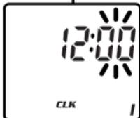
**Step 3:** To set the current time, press Button #2 to advance the flashing digit, then press Button #1 to select it and advance to the next flashing digit.
