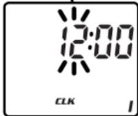
**Step 2:** Press Button #1 to select the desired time format and advance to the Clock Setup screen with the left hours digits flashing.
