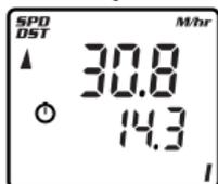
The V100A can be calibrated for two bicycles. It will store separate Wheel Size, Service Timer, Odometer and Altitude settings, as well as different formats selected for Time, Temperature, Speed and Distance. The current bike number (I or II) is always displayed in the lower right corner of the screen. To switch the computer quickly from Bike I to Bike II, go to the first screen in the Normal Operating Mode Setup program. (See SETUP section below for details.)
