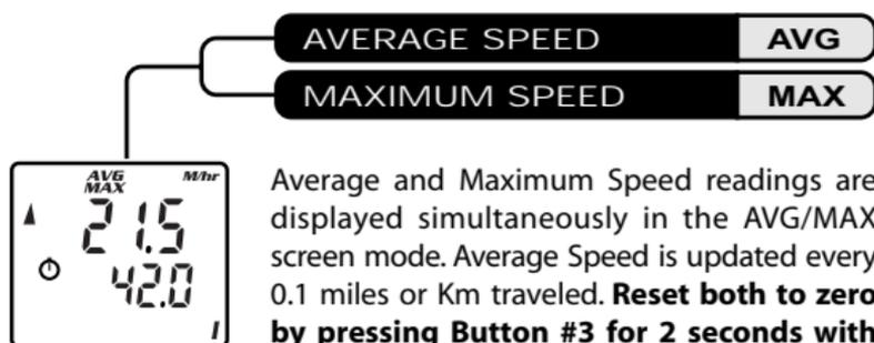
Average and Maximum Speed readings are displayed simultaneously in the AVG/MAX screen mode. Average Speed is updated every 0.1 miles or Km traveled. **Reset both to zero by pressing Button #3 for 2 seconds with timers turned off in any screen mode except STP/ID or STP/IA.**
