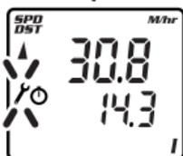
Alerts rider when Ride Time reaches a preset limit for a maintenance check on the bike or any main component. Suspension forks, rear shocks, chains, etc. require service at specific time intervals set by manufacturers. Vetta's Service Timer allows the rider to preset an exact number of riding hours during Setup, then signals (slow, flashing wrench icon) when the service time limit has been reached. (See SETUP section below for details.)
