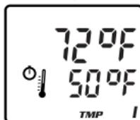
To display both the Maximum and Minimum Temperature readings, press and hold Button #1 for 2 seconds in the Temperature SPD/TMP screen mode. **Note:** The screen will flash to indicate that the computer is displaying data in a secondary screen. To return to the primary SPD/TMP screen mode, press Button #1 again. When ride data is reset by holding Button #3 with the timers stopped, both Maximum and Minimum Temperatures reset to the current Temperature.
