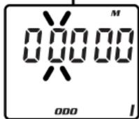
Bike I and Bike II have separate, programmable odometers. On a new computer the Odometer screen should read "00000" for both. To confirm this initial zero setting, simply press Button #1 successively to select each flashing digit and advance to System Check. To reenter mileage achieved after a battery change, follow these steps:
