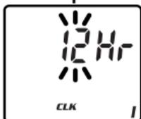
The V100A clock displays time in either a 12 or 24 hour format. A "PM" indicator appears only in the 12hr format. To select a format and set the current time, proceed as follows:
