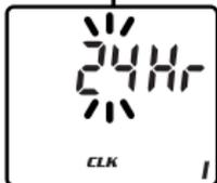
**Step 1:** Use Button #2 to toggle between the two time formats (the numbers will flash).
