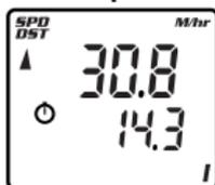
SPD displays the current Speed and is updated continuously. DST displays the current Trip Distance and automatically resets after the maximum trip distance (999.9) is achieved. Trip distance is displayed in the SPD/DST screen mode and starts automatically when the wheel rotates and TT Timer is active. **Reset DST to zero by pressing Button #3 for 2 seconds with the timers turned off in any screen mode except STP/ID or STP/IA.**
